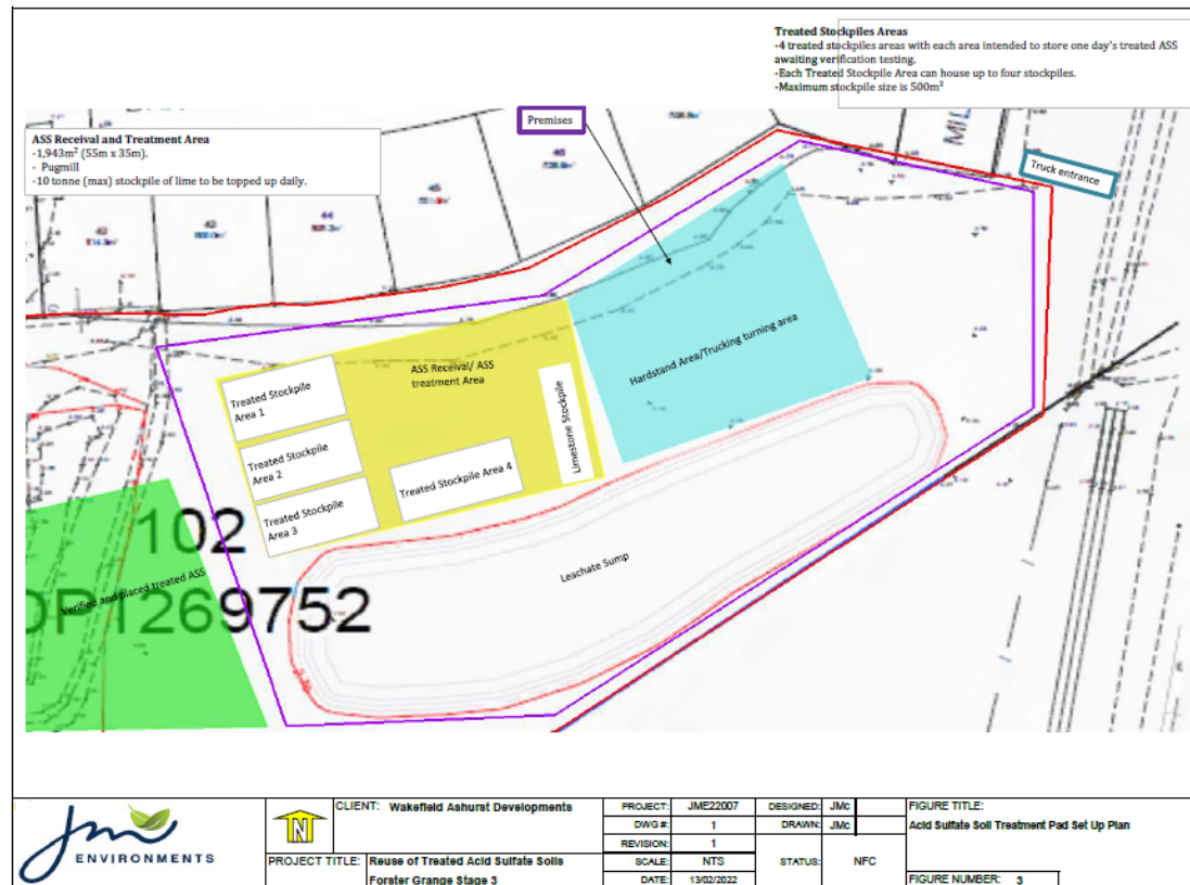
Figure 3: ASS Treatment Pad set up Plan
